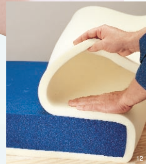
For easy bullnose fabrication in a compound cushion, 3M™ Fastbond™ Foam Adhesive 100 bonds a lighter density foam around a higher density core. High tack holds in seconds.
