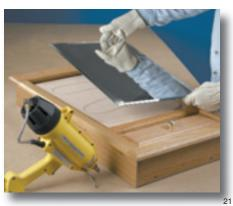
Long open time provides production speed flexibility for bonding a mirror to plywood or MDF panel in a medicine cabinet door.
