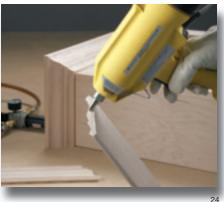
With a thin bond line, PUR 250 adhesive makes a secure, aesthetically-pleasing crown molding assembly.
