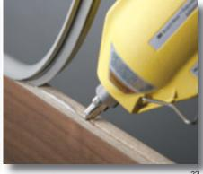
A neatly applied bead of adhesive bonds the extruded plastic edge molding to the particle board core of a counter top.
