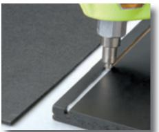
Permanently and quickly bond wood and MDF (Medium Density Fiberboard) bottoms and side panels in drawers.
