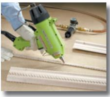
For both PUR Easy and PUR Easy 250, an optional filter/pressure regulator is available to remove particulate material and water.
