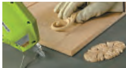
Bond simulated-wood plastic trim to wood cabinet doors with an invisible bond line.
