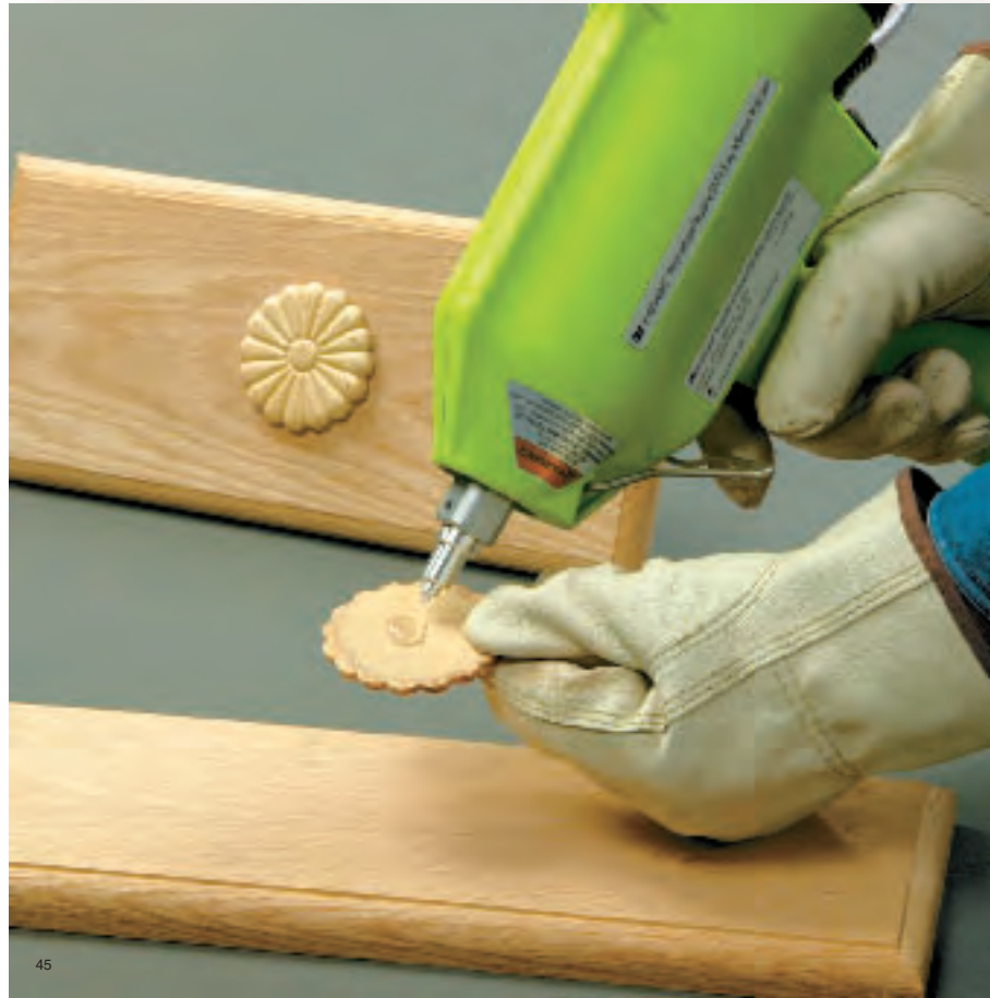
Bond wood or plastic rosettes to wood drawers without fixturing or drying time. Adhesive dispenses warm at 170°F (77°C) and can remain in the applicator at dispensing temperature for up to 40 hours.
