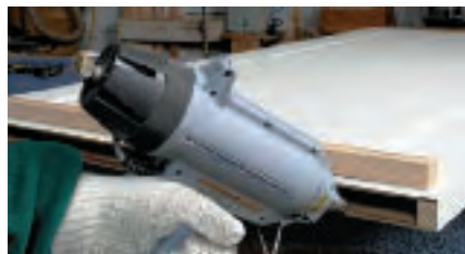
37 To increase production, 3M™ Scotch-Weld™ Polyurethane Reactive (PUR) Adhesive System bonds fir reblock strips between hardboard door panels. Also improves the bond between weather stripping and a vinyl extrusion.
