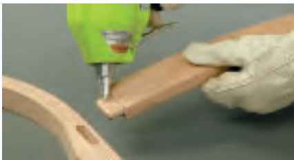
Trigger a fast, easy, and neat bead of adhesive from self-contained hand-held applicator at up to 11 pounds per hour.
